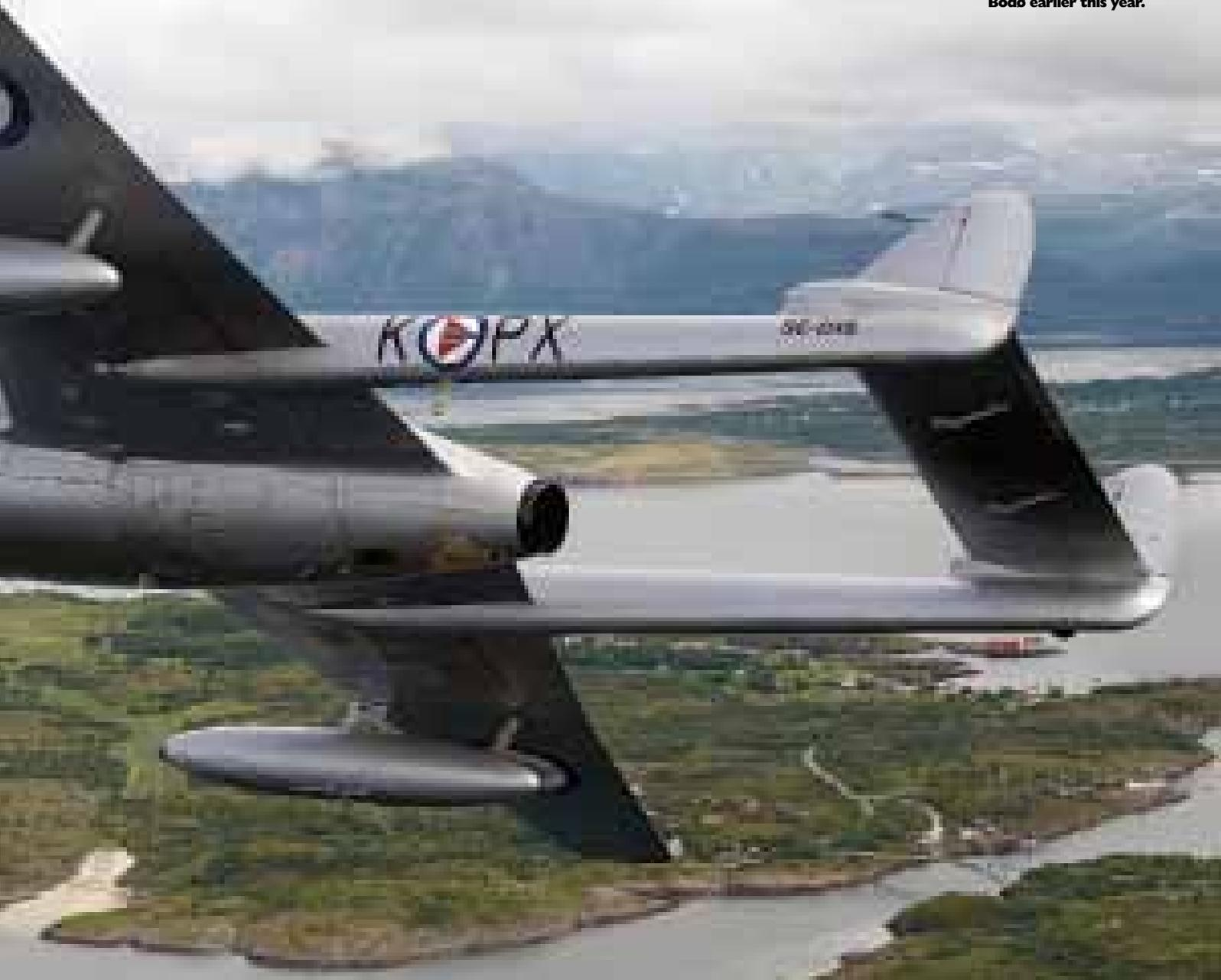
T55s, using the type for air defence, ground attack and advanced training. Weaponry included four 20mm Hispano guns, two 500lb bombs and unguided rockets.
